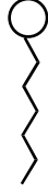
Figure 1.3: A typical lyotropic molecule, with a polar head and a nonpolar tail.
